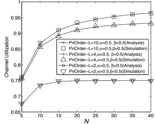
Fig. 7. Channel utilization with different number of S-D pairs
