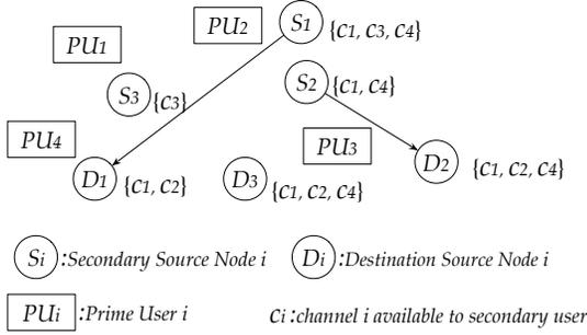
Fig. 1. A cognitive radio network with heterogeneous channel availabilities at different secondary nodes.
