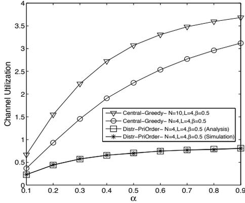
Fig. 5. The comparison of centralized and distributed algorithms
