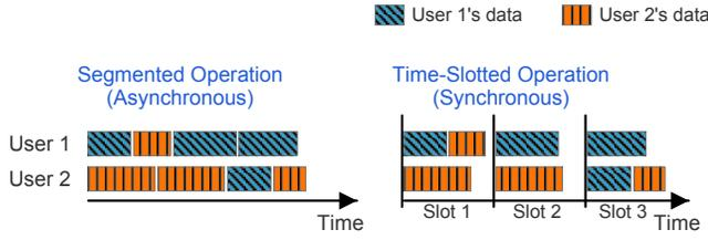
Figure 3. Segmented vs Time-Slotted Operation.
